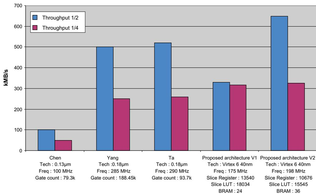
**Fig. 4.** Comparison of the FME architectures throughput performances.
