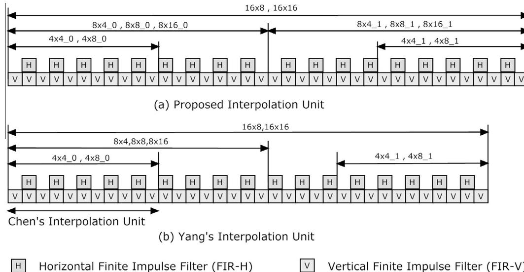
Fig. 3. Half-pel interpolation units.
