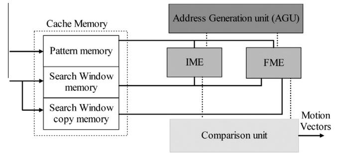
Fig. 1. The top-level view of the proposed motion estimation architecture.
