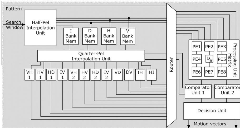
Fig. 2. Overall FME architecture.
