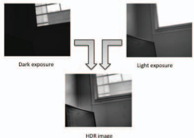
Fig. 1. Multiple exposures combined into one HDR image
